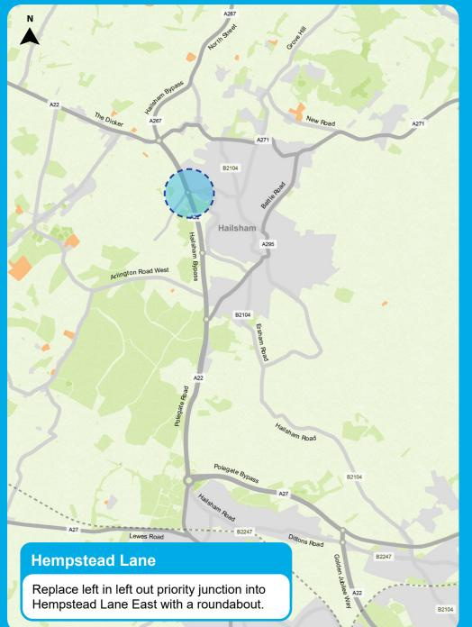
The proposals are to replace the priority left in left out junction with a roundabout. This allows movements from all approaches to travel in every direction - not possible with the existing layout. A signalised Toucan crossing is proposed on the southern arm of the junction. The speed limit would need to be reduced to 40mph.
